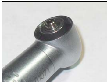
3 Insert turbine assembly into head housing
