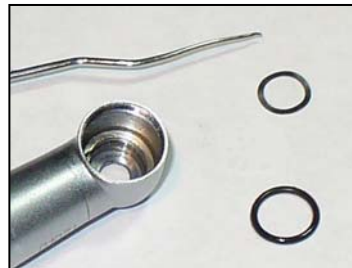
2 Place 3-point washer and o-ring into head housing
