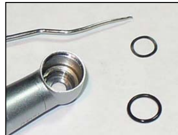
2 Place 3-point washer and o-ring into head housing
