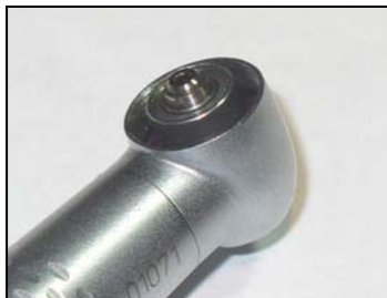
3 Insert turbine assembly into head housing
