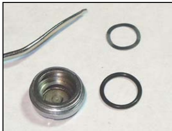
1 Place 3-point washer and o-ring into back cap
