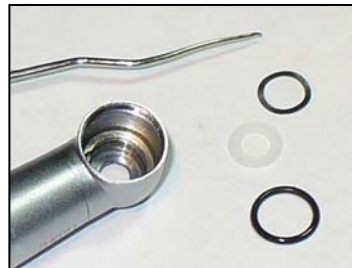
2 Place 3-point washer, plastic washer, o-ring in head housing
