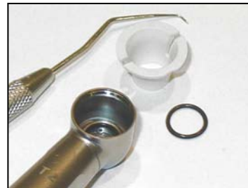
2 Place o-ring into head housing using insertion tool
