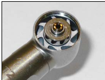
3 Insert turbine assembly into head housing
