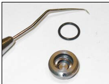
1 Place o-ring into back cap
