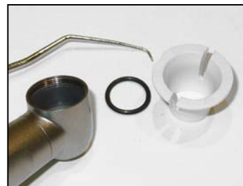
2 Place o-ring into head housing using insertion tool
