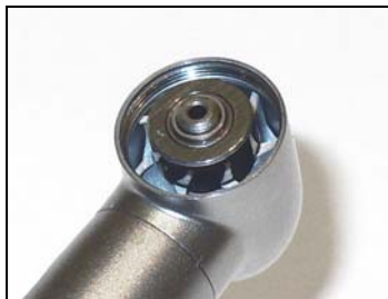
3 Insert turbine assembly into head housing
