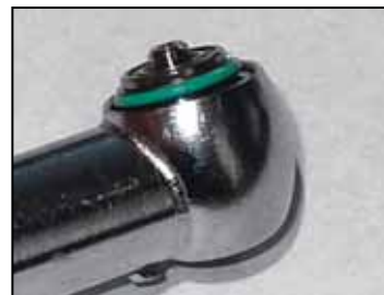
2 Insert turbine assembly into head housing
