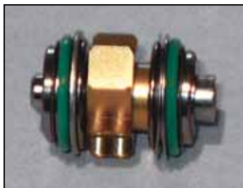
1 Verify o-rings are seated on front and rear bearings of TA
