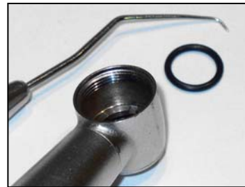
2 Place o-ring into head housing
