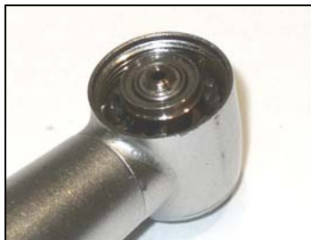
3 Insert turbine assembly into head housing
