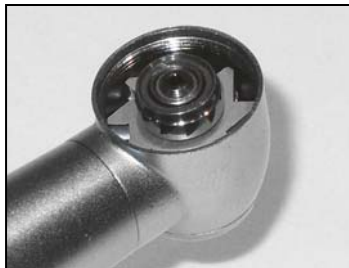
3 Insert turbine assembly into head housing
