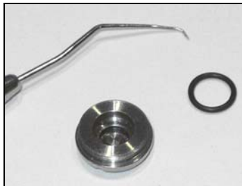
1 Place o-ring into back cap
