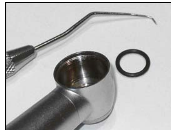
2 Place o-ring into head housing
