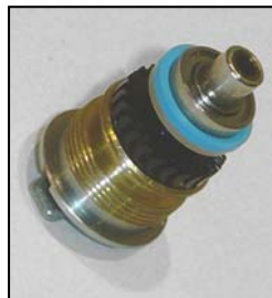
3 Insert TA into back cap
